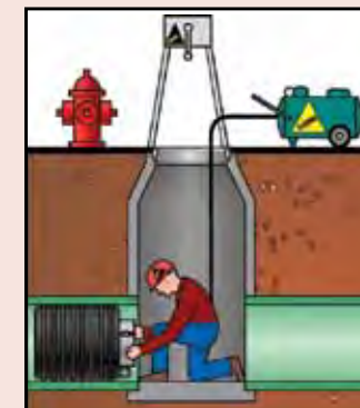
1) Install plug to isolate manhole
